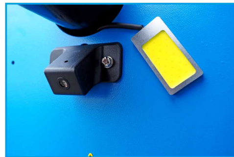
LASER POINTER / INNER WHEEL LIGHTING
