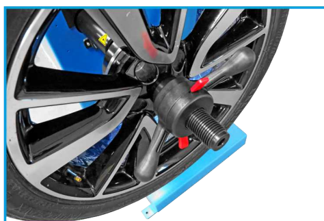
NUTRUNNER IN A BALANCER WITH A CLUTCH
