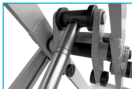
INITIAL LIFT PHASE SUPPORT SYSTEM
