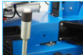
Push-button controlled bead breaker
